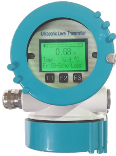
“UPC-LT-330” level type ultrasonic transmitter is a level measurement device best suited for storage tanks it has a local display with buttons for quick and easy commissioning. Temperature compensation is integrated and can be equipped with an external sensor for dynamic temperature compensation. the automatic false echo detection together with easy set up makes it reliable and trustworthy.
